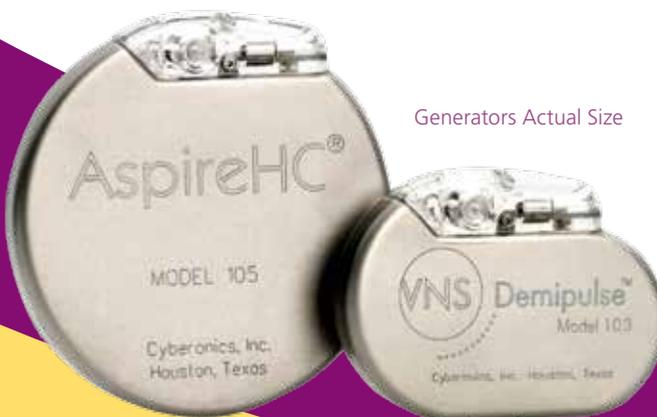
A small generator about the size of a watch is placed under the skin usually in the left chest area. A thin, flexible wire connects the generator to the left vagus nerve under the skin in the neck.
